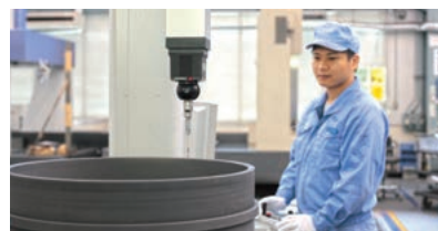
Inspection using 3D measurement machine
